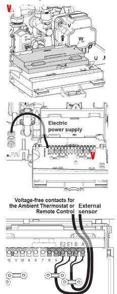
Unscrew "V" and lift the cover "W" to access the electric power supply terminal block, remote and external sensor
