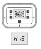
2) Press C once, the display shows Par (Parameters Menu), then press B to enter the menu
